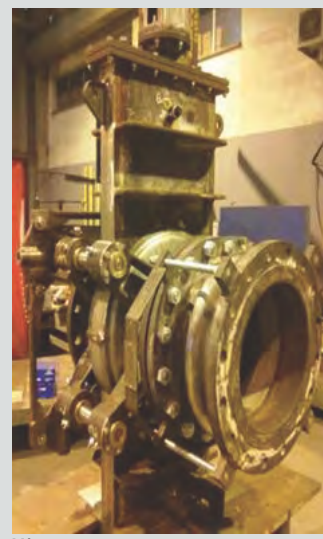
VÁLVULA OCULAR TIPO LINEAR ENCLAUSURADA MANUAL – VERTICAL GOGGLE VALVE WITH ENCAPSULATION, LINEAR AND MANUAL - VERTICAL
