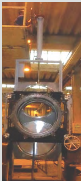
VÁLVULAS OCULAR TIPO LINEAR SEM CLAUSURA MANUAL – VERTICAL GOGGLE VALVE WITHOUT ENCAPSULATION, LINEAR AND MANUAL - VERTICAL
